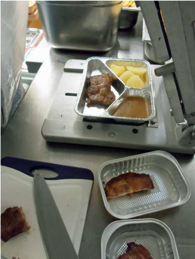
Picture: Filling and seaming of aluminium foil containers
