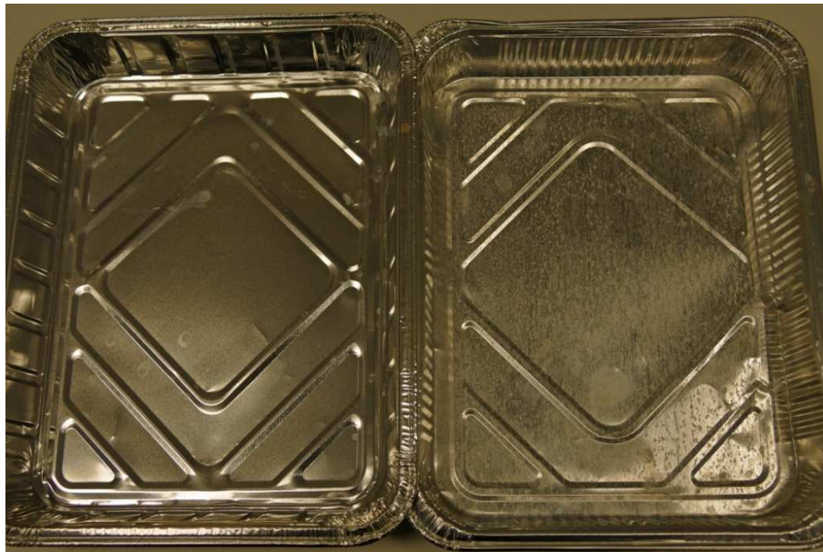
Picture: Foil containers after contact with foodstuff sample no.14: foil container 1.1. (left) no visible corrosion defects and foil container 2.1 (right) with corroded internal surface
