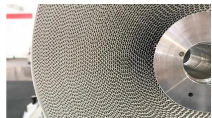
The aluminium foil is chemically degreased and lacquered both sides with the hygroscopic formulation and anticorrosion primer. The formulation is applied through coil coating. An additional benefit is a reduction of the flow rates of refrigerant fluid, which also contributes to higher efficiency of the rotor.
