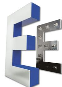
The aluminium foil replaces wired assemblies. The PowerBoard is a recycled PET panel, laminated with three layers of aluminium alloy AA 1200 and the wireless LED lights are just screwed anywhere into the surface. The layers of aluminium foil are excellent conductors of electricity and enable the modules, or letterboxes, to be made in many intricate shapes and sizes, quickly and with the potential of using automated assembly methods.
