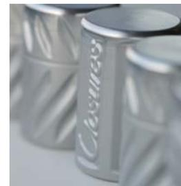
The **Imagic** uses Electro Magnetic Forming (EMF), first developed for military use, to create almost any shape, including round, pyramidal and precisely decorated. The effect is achieved by placing an aluminium shell over a plastic 'skeleton' or mould. Using EMF the shell takes the shape of the mould. The finished product is very resistant and so avoids dent problems, both during production and transportation. The closures combine the functionality of plastics with the aesthetics of aluminium.
