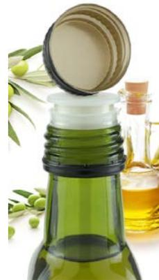
An integrated 'No-Touch' system enables hygienic opening and handling, while the flow control within the insert allows for precise pouring. The drop-cut system means both the bottle and label stay clean as the excess liquid is captured and returned to the bottle. Also the combination cap incorporates an anti-refill device within the HDPE system while the aluminium element includes a tamper-evident band.
