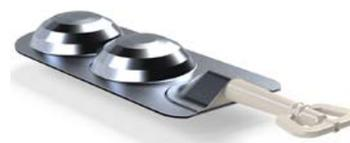
The blister was jointly developed with machine builder **Rohrer - Leading Solutions**. One chamber is filled with a dry powder incorporating the active ingredient (highly moisture-sensitive), the other one with a liquid. Thanks to the peelable frangible seal which opens the channel, both components are mixed by pushing on the cavities.
