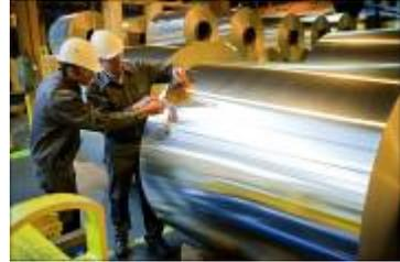
Aluminium foil has a unique combination of properties including barrier, deadfold and formability which have made it an essential part of many flexible packaging and container applications. Other uses of aluminium foil include automotive and heat exchange components, insulation material and many industrial applications.
