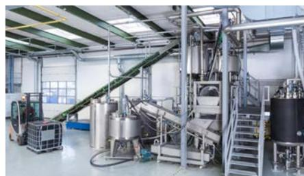
saperatec's process can delaminate polymer and metal films, then separates each into secondary raw materials for recycling
