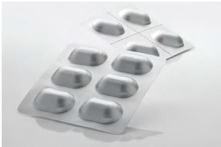
The base foil is a multiple layer laminate with a core of 45µm thick alufoil. The lid foil is made from alufoil of 25µm thickness, lacquered on both sides. Together they provide a complete barrier against moisture. In the new blister design the perforations between the single cavities have been removed, improving the resistance to moisture diffusion considerably. Also this has enabled six tablets, rather than the previous four, to be packed in a blister with identical dimensions. ///
