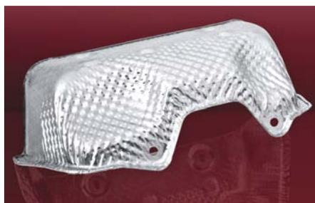
parasitic noise and the risk of high cycle fatigue failure. The new 'sandwich' foil material, comprised of 0.2mm alufoil/0.08mm polymer/0.3mm aluminium strip, effectively damps the vibration and reduces the risk of fatigue cracks. Noise emission is completely eliminated so the overall environment in the vehicle is greatly improved. ///
