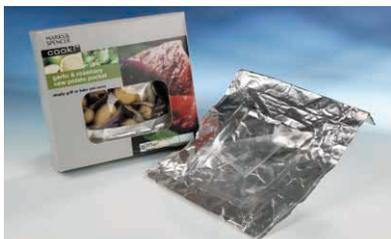
The product is visible to the chef during cooking and the pack expands to provide a 'chamber' that self-vents to allow pressure and steam to escape safely. The easy-peel polyester window allows good product visibility, while tailored oxygen permeability supports extended shelf life for products.
