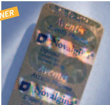
20 µm alufoil blister pack material is used, and the special Aventis hologram surface design does not affect its machinability.
