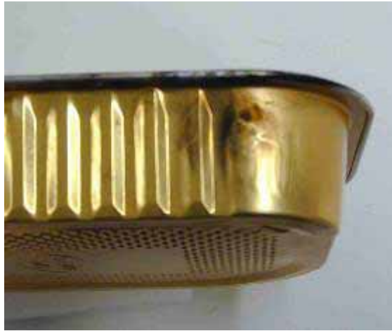
Figure 6.11: Aluminium foil tray after touch with cooking chamber wall during microwave exposition.
