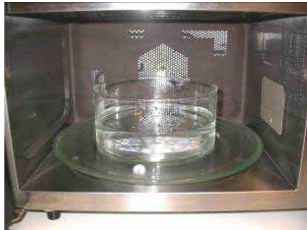
Figure 5.5: Arrangement of 1 l water in container for measurement of actual oven power
