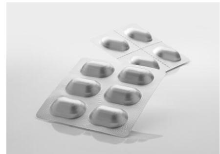
The base foil is a multiple layer laminate with a core of 45µm thick alufoil. The lid foil is made from alufoil of 25µm thickness, lacquered on both sides. Together they provide a complete barrier against moisture.
