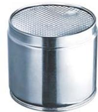
When filled and stacked, pressure is applied only to the outside rounded seam; no force is exerted on the SealLite® membrane. The design of the lid and can also increases the fill volume for the product.
