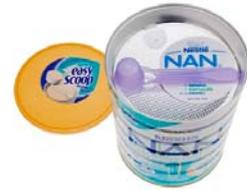
Easy Scoop features a combination of a new Deep Drawn End from Ardagh Group utilising an Alufix® Dry Pro peel-off alufoil membrane from Amcor Flexibles Singen. The pack creates a cavity for a spoon by sealing the bottom of the steel deep drawn end with the alufoil membrane to the inner part of the ring. The end is sealed to the can in the normal way, and the pack is topped by a plastic lid.
